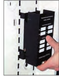
Step 3 - Push cover on module
